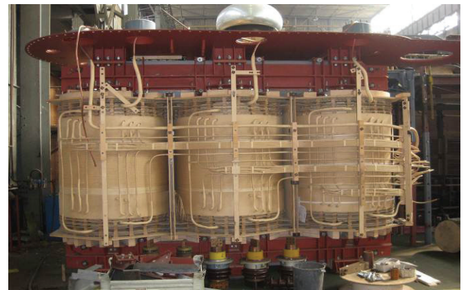
Fig. 11 The active part of power transformer
