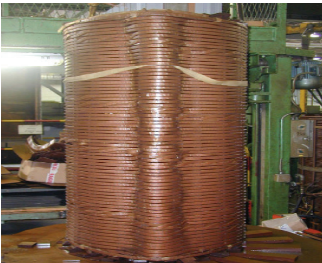
Fig. 13 Deformation of windings due to short circuit
