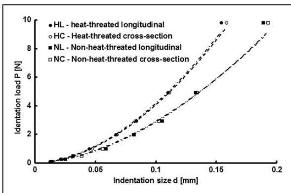
**Figure 4.** Indentation load versus indentation size according to the Meyer's law.
