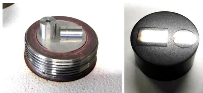
Fig.5 Sample preparation for micrographies, in particular the resin embedded sample (longitudinal and cross sections) is depicted on the right
