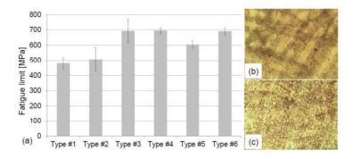
Six sets of specimens have been manufactured according to ISO 1143 for fatigue tests under rotating bending. In particular, they have uniform section at gage and they have been loaded under four-point bending. The six sets can be regarded within
