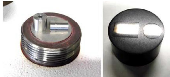
Figure 9. Specimen preparation for micrography
