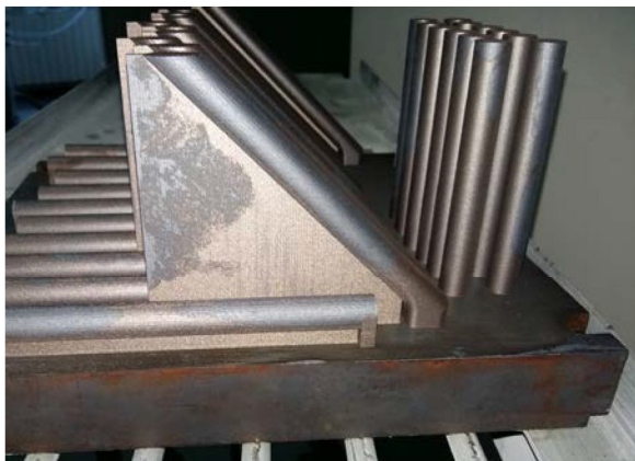
Figure 5. Samples position and orientation in working volume on EOS M 280
