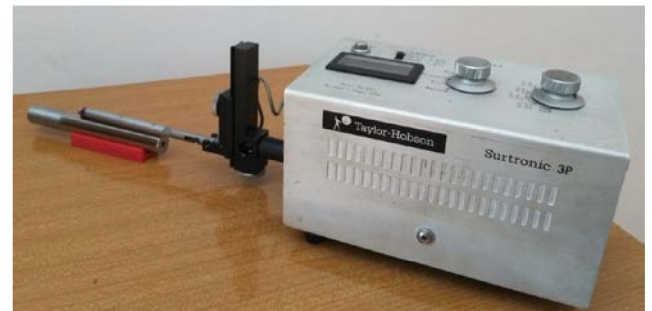
Figure 7. Taylor-Hobson Surtronic 3P for measurement of the surface roughness
