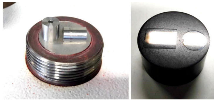
Figure 4. Sample preparation for micrographies, in particular the resin-embedded sample, (longitudinal and cross sections) is depicted on the right.
