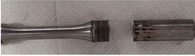
Figure 4: Unexpected failure at sample head
